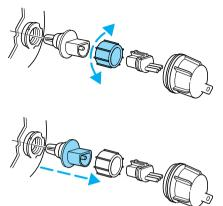
6. Without turning, remove the old bulb from the lamp assembly by pulling it straight back out of the lamp assembly and replace.
